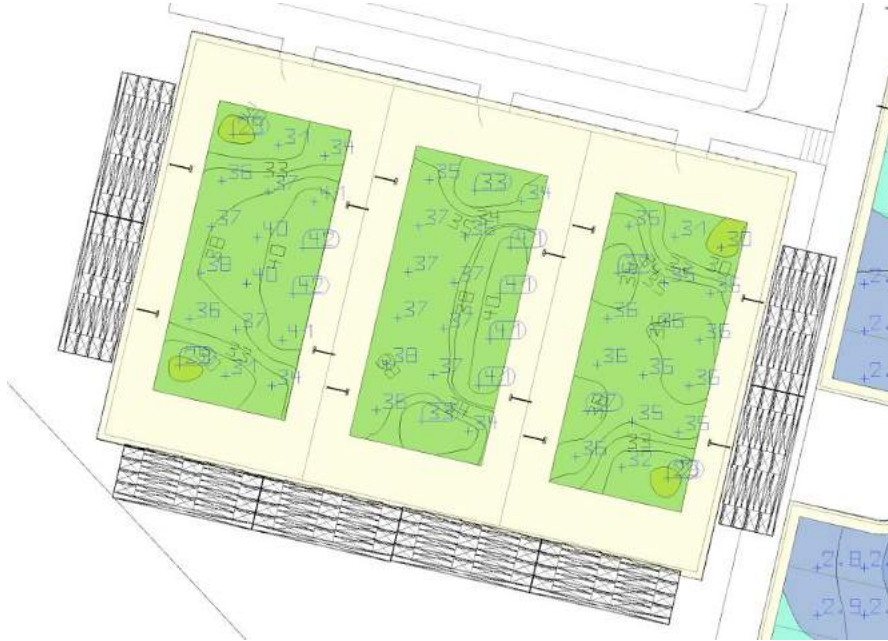
RET Photometric Results using 135-watt fixtures and 120 Ah batteries.
